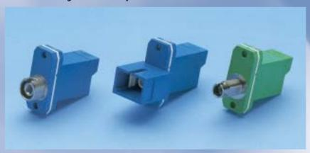
E-2000™ Hybrid Adapters allow connections between the E-2000™ connector and FCPC, FLSA or FSC connectors. All Hybrid Adapters are equipped with a slotted zirconia ceramic sleeve. The adapter operates at temperatures between -40°C to +85°C.
