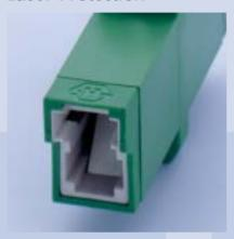
The integrated full-metal diaphragm in the adapter protects from emerging laser light. The full-metal safety cap in the connector opens and closes automatically. The safety cap has an integrated spring safety device which prevents the ferrule end faces from becoming dirty or damaged.
